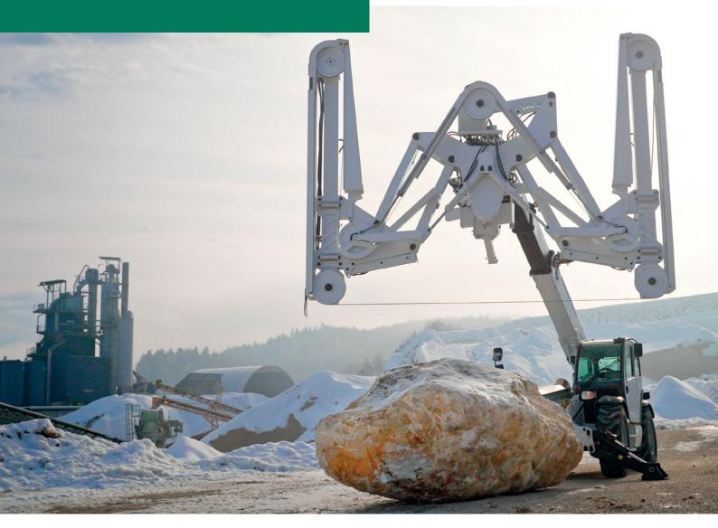
Cutting width < 5 mCutting depth < 3.4 m
